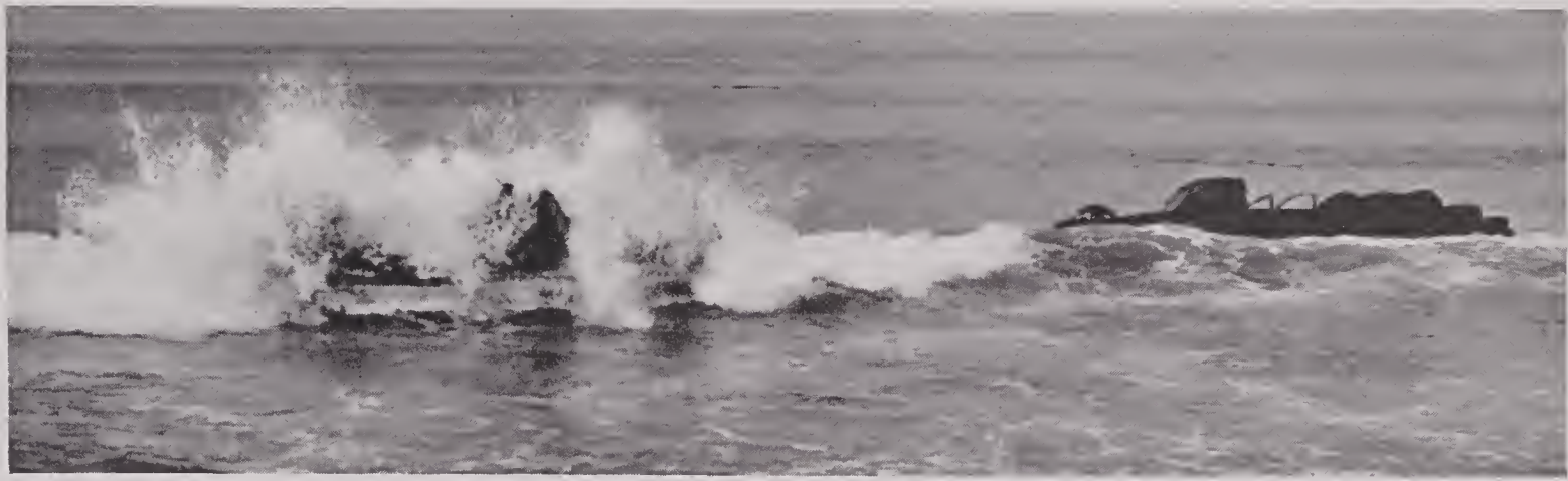
FIGURE 54. DUKW surf ability tested in moderate surf at Monterey Bay, California.
